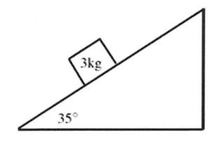
The diagram on the left shows a box of mass 3.00 kg sliding down a ramp inclined at  $35.0^{\circ}$  to the horizontal, against a constant 10.0N frictional force.
