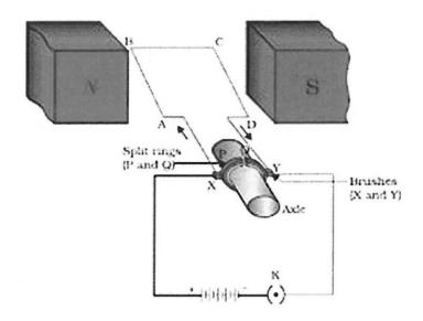
The diagram on the left represents an electric motor with a rectangular coil containing 425 loops. Each loop has two long sides (AB and CD) which are 9.50cm long, and has a width (BC) of 5.25cm. The current flowing through the circuit is 1.25A and the magnetic field intensity is 0.455T.
