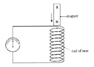
The diagram on the left shows a bar magnet about to fall through a coil of wire.
