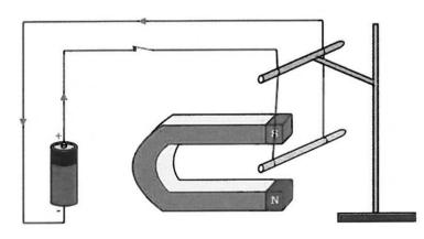
The diagram on the left shows a metal rod carrying a current of 0.560A, in a uniform magnetic field of 0.0540T. The uniform field extends along 13.5cm of the metal rod. The wooden retort stand on the right of the diagram has a horizontal wooden bar designed to hold the wires away from the magnet.
