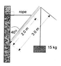
The diagram on the left shows a system in static equilibrium. The 3.00m long uniform beam has a mass of 12.5kg and supports a mass of 15.0kg from its end. It is hinged to the wall of a building, making an angle of 40.00 to the vertical. The beam, in turn, is supported by a rope that is joined at a point 2.00m from the hinge, and makes a perfect right angle with the wall.
